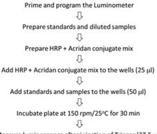
Measure luminescence after injection of Trigger (37.5 µl)
